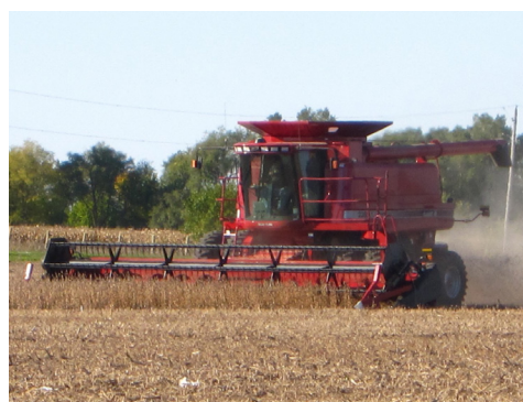
Figure 1. Most mechanical seed loss or seed shattering occurs at the gathering unit, between the header and standing soybean plants.
