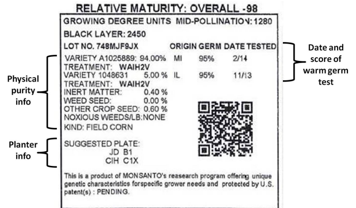
Figure 2. Quality control information contained in seed tags includes the seed lot number, physical purity scores, and the date and score of the warm germination test. Also included are planter recommendations for the specific seed type.
