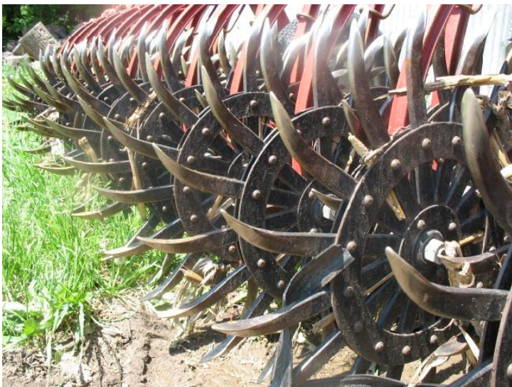
Figure 4. A rotary hoe consisting of dozens of finger-like tines made to disturb the soil surface.
