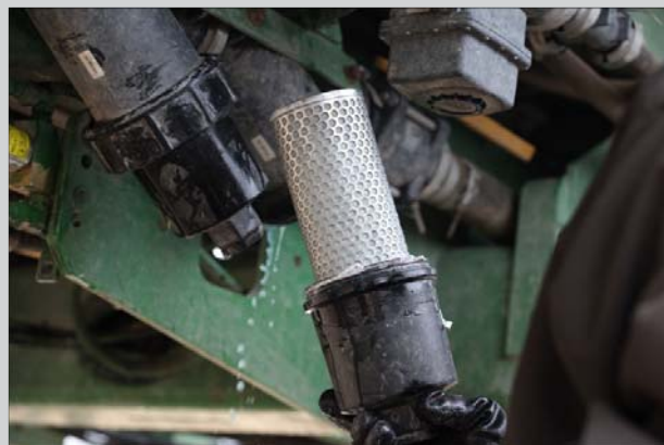
Figure 1. Filters and screens should be cleaned to remove residues.
