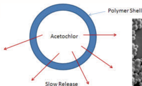
Figure 1. Diagram illustration of micro-encapsulation technology and electron microscope picture showing microcapsules of Warrant® Herbicide.
