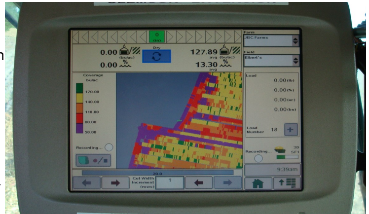
Figure 1. Without proper calibration, yield monitor data does not provide a reliable picture of crop yield.
