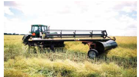
Figure 1. Swathing canola with a roller. Photo courtesy of M. Stamm, Kansas State University.
