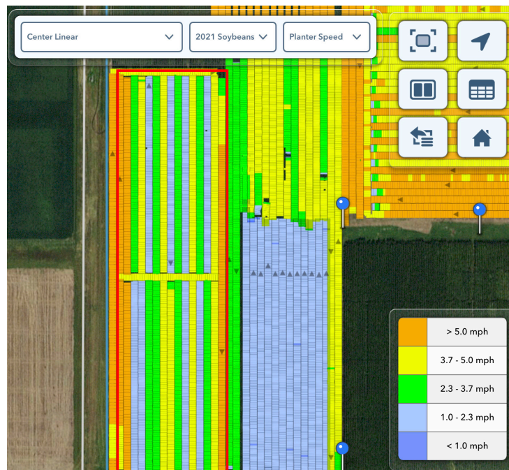
Figure 1. Speed of planter passes as reported in Climate FieldView™. The plot area is highlighted in red.
