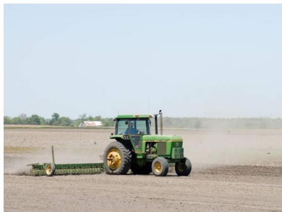
Figure 2. A rotary hoe can be an effective tool for fracturing crusted soils.
