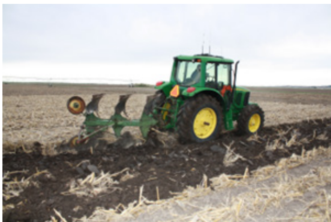
Figure 1. Moldboard plow at Bayer Learning Center, Gothenburg, NE. Where appropriate, moldboard plowing can bury weed seed below germination levels.
